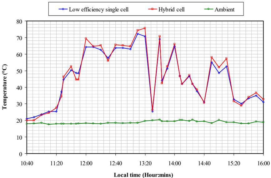
Figure 9 shows the variations of operating cell temperatures and ambient temperature over the experimental test period during a partial cloudy day. It can be seen that both PV cells had almost the same operating temperatures, which means that the observed differences in power output between the PV cells (Figure 8) was not due to their differences in operating cell temperature.
