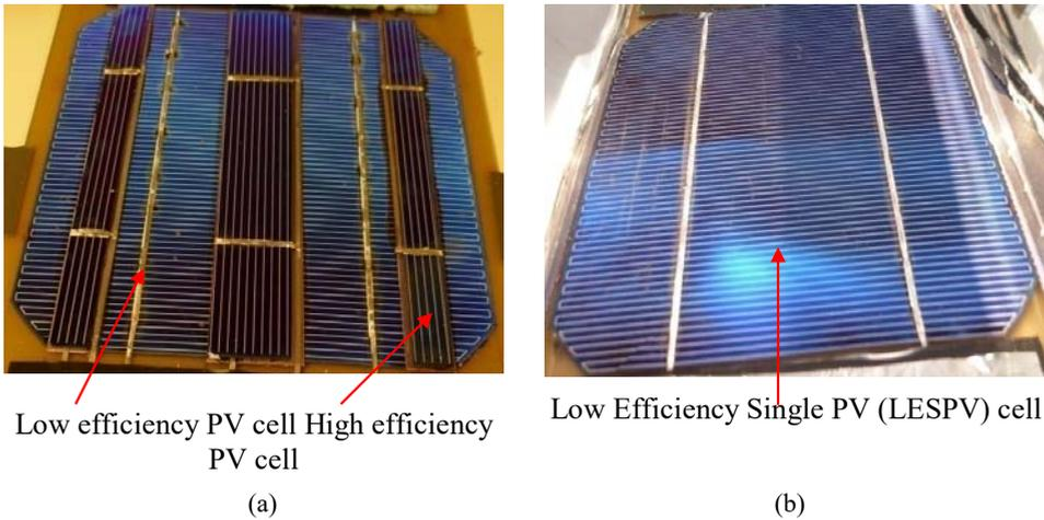
For direct comparison with a hybrid PV cell, LE single PV (LESPV) cell was also fabricated. Figure 4 shows the photographs of the two fabricated PV cells.
