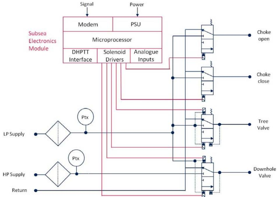
The SCM consists in principle of a pressure and temperature compensated, dielectric oil filled chamber, bound by a protective cover and baseplate. Within the dielectric chamber are housed all major hydraulic and electrical components. Incoming electrical supplies are provided via two electrical connectors located at the top of the unit. Hydraulic connections are made via couplers located in the baseplate of the SCM and hidden from view in normal operation by a protective skirt.
