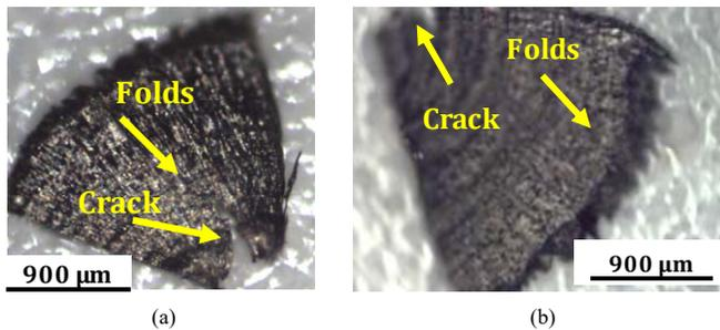
**Figure 10** Surface topography of the face milled nickel alloy 625 fabricated via LPBF ( $v_c = 90$  m/min,  $f_z = 0.1$  mm/tooth, case 1), (a) digital optical image (b) scale-limited surface (c) scale-limited areal surface topography (see online version for colours)
