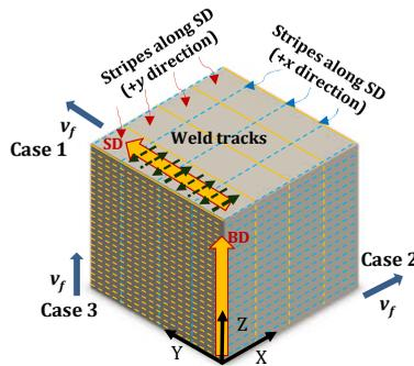
The influence of scan strategy (or stripe pattern) rotation on the machinability of the LPBF nickel alloy 625 was also investigated. Two workpieces with different scan strategy rotations were used in this work; a workpiece built with scan strategy rotation of  $90^\circ$ , and another one built with  $67^\circ$  rotation. Both workpieces were face milled by following climb milling engagement in three cases as indicated in Figure 3.
