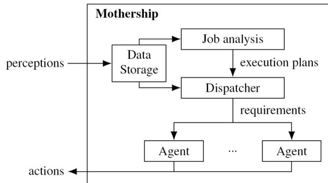
The general structure of the framework is shown in Figure 1. The user configures the application via a command-line interface, which in turn calls the session manager, to handle the necessary state of a connection with MASSim over multiple simulations. The session manager relies on the message subsystem to communicate with MASSim over a TCP/IP socket. It instantiates a Mothership for each simulation and transfers the perceptions and actions between the Mothership and the message layer.
