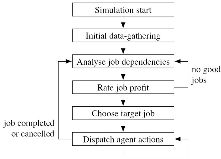
Thus, we have three components: the job analysis to build the dependency tree, the dispatcher, which executes this tree by assigning requirements to agents, and the finite state machines that execute the requirements, yielding the actions for the agents.
