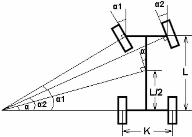
In Figure 2,  $\alpha_1$ ,  $\alpha_2$  and  $\alpha$  are command of turning angle of left front wheel, turning angle of right front wheel and turning angle of steering plate respectively,  $K$  is nodal distance of left and right steering,  $L$  is axle distance of front and rear wheel. Formula of turning angle deduced from figure is as follows:
