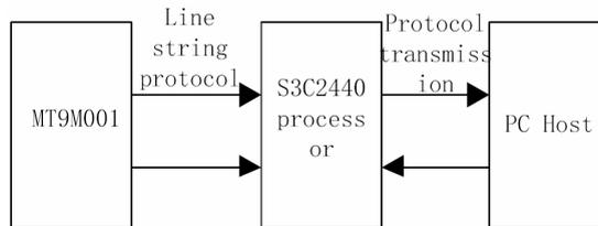
It can be seen from Figure 1, the system followed the string transmission protocol. It used MT9M001 model sensor to transmit frame data, line data and pixel data to the S3C2440 processor. It went through the processor for related big data processing, transformation and fusion, and transmits data to the image processing host through protocol transmission. Based on this principle, the system hardware and software were designed.
