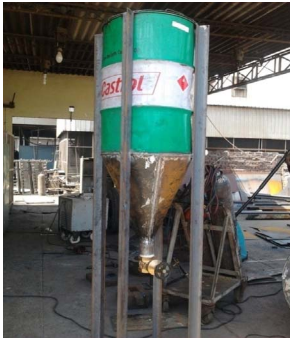
Figure 13 Centri-gravitational equipment under construction (see online version for colours)
