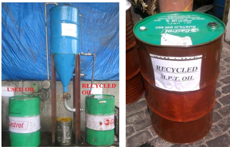
Figure 14 Centri-gravitational equipment in working and recycled M.P.T. oil drum (see online version for colours)
