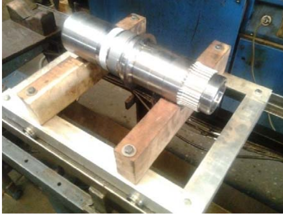
Figure 7 First change in trolley those wooden blocks (see online version for colours)
