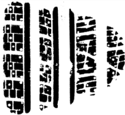
Figure 1 Footprint on a flat surface of Pirelli Scorpion Verde 235/55 R19 105V tyre at -4^\circ camber at 250 kPa inflation pressure
