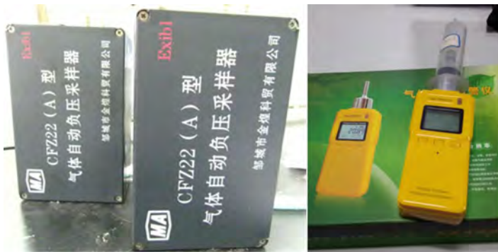
Figure 6 Negative sampling pumper devices and methane concentration diameter (see online version for colours)
