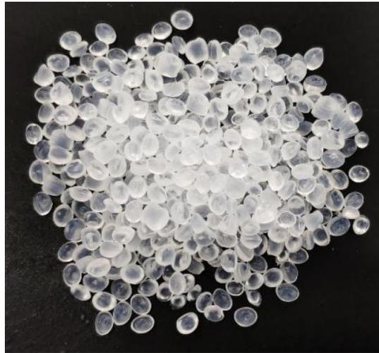
In this paper, EVA particles were selected as asphalt modifier, which contained 15% VA content, with a diameter of about 0.5 cm. EVA particles were produced by YUCHENLONG engineering plastics company (see Figure 1). The physical properties of EVA plastic particles were shown in Table 2.
