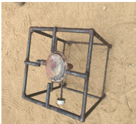
Figure 5 Valve modified stove for biogas use (see online version for colours)
