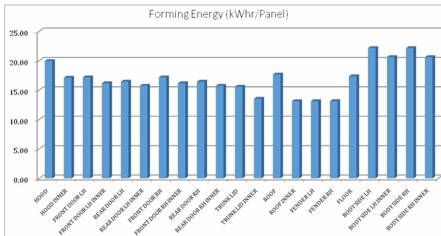
Combining the panel forming model with the look-up macro into a unified code can provide useful insights on the automotive manufacturing energy break-down, as displayed in Figure 5(a) and the energy type in Figure 5(b). Such analysis reveals processes or practices that should be targeted for energy saving efforts. From this study, a complete steel BIW will consume around 600 kWhr/vehicle, while a complete Al BIW consumes around 820 kWhr/vehicle.
