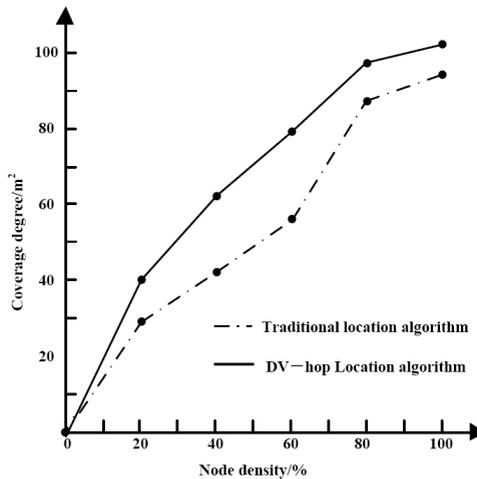
Figure 5 is an analysis graph of positioning coverage (%) based on a DV-hop positioning algorithm and a conventional positioning algorithm. As can be seen from the figure, when the node based on the DV-hop algorithm is located at the anchor point rate less than
