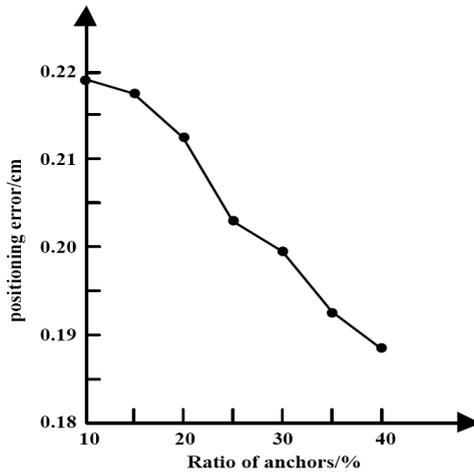
Figure 6 is a diagram showing the relationship between the change of the anchor ratio and the positioning error (cm). As can be seen from the figure, as the proportion of anchor points increases, the positioning error decreases. When the anchor points are
