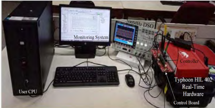
Figure 6 Hardware-in-the-loop experimental setup (see online version for colours)
