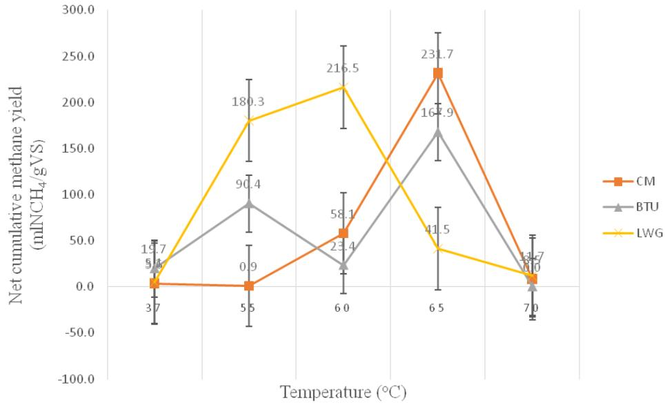
**Figure 3** Comparison of net normalised cumulative volume of methane content for three inocula at optimal temperatures of 37°C, 55°C and 65°C (see online version for colours)
