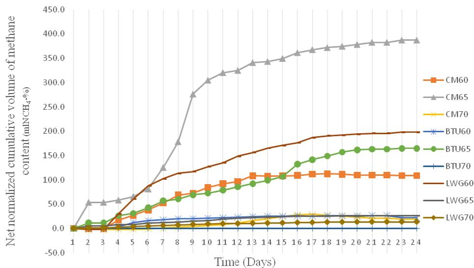
**Figure 2** Comparison of net normalised cumulative methane yield for three inocula at hyper-thermophilic temperatures and optimal mesophilic temperature of 37°C and thermophilic temperature of 55°C (see online version for colours)
