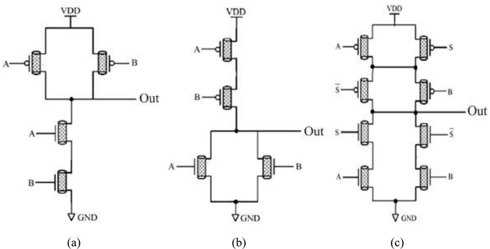
**Figure 2** (a) CMOS-based NAND gate, (b) CMOS-based NOR gate, (c) CMOS-based MUX and (d) CMOS-based XOR gate (continued)
