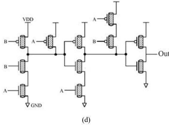
**Figure 3** (a) CPL-based NAND gate, (b) CPL-based NOR gate, (c) CPL-based MUX and (d) CPL-based XOR gate
