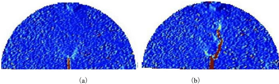
**Figure 9** Failure diagram of dynamic SCB test specimen at different wavelengths, (a) 100  $\mu\text{s}$  (b) 300  $\mu\text{s}$  (c) 900  $\mu\text{s}$
