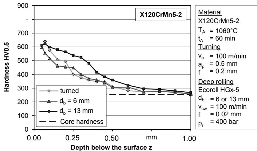
In order to improve the transformation behaviour of the special alloy X120CrMn5-2, an adaption of the preliminary heat treatment was carried out by varying the austenitising temperature  $T_A$ . Thereby, the microstructure of the material was adjusted to ensure a change in the stability of the austenite and also modified transformation behaviour.
