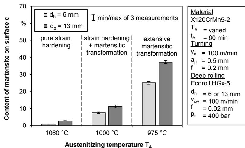
These results are also confirmed by the magnets-inductive measurement of the content of martensite at the surface of the special alloy under the varied microstructural stability (Figure 10). By lowering the austenitising temperature, the microstructure of the material becomes more instable, so that an increased martensitic transformation is recorded.
