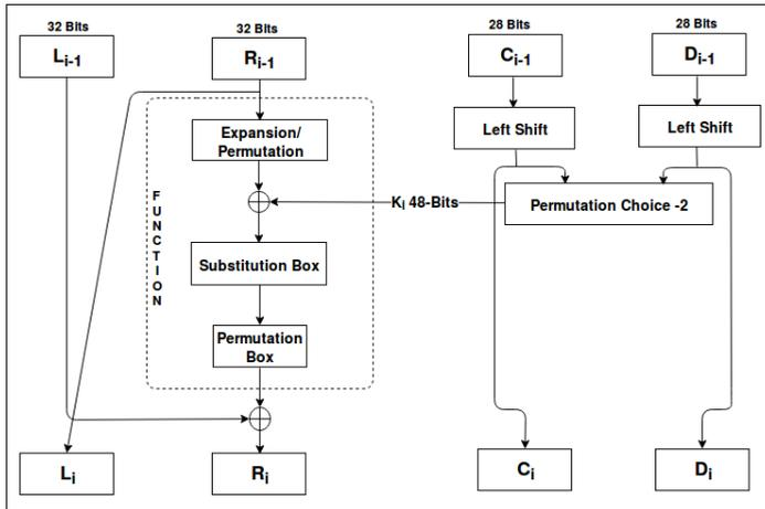
After IP, the plaintext is divided into  $L$  and  $R$ . This  $R$  becomes new  $L$  of the next round and new  $R$  is the x-or of the previous round  $L$  and output of the  $F$  function. The whole process can be explained by the following equations:
