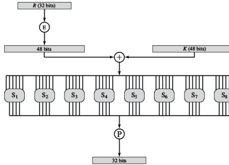
The expanded 48 bit output is xor-ed with 48 bit key and given as input to the eight s-boxes each of which takes 6 bit as input and gives 4 bit output. So this 48 bit xor-ed output is divided into eight blocks of 6 bit each and each of them is given as input to the s-boxes. These 48 bits get transformed into 32 bits as four bit output is obtained from each s-box.
