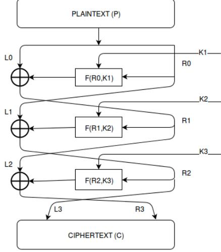
$R'_3$  is the xor-ed difference of  $R_3$  and  $R_3^*$ . So,  $R'_3 = R_3 \oplus R_3^*$ .
