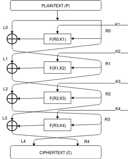
Even though we can have a probability characteristic with better probability like  $p = 1/2$  or  $p = 1$ , we are not using such characteristic so that we can have  $R'_1 = 00000000$  which expands to be all zeros. This helps us in getting key bits entering all eight s-boxes. That is we can get 48 bits of key.
