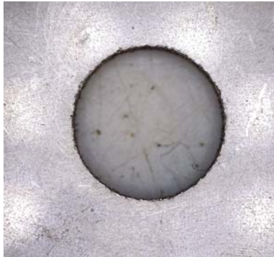
Figure 4 Machined hole using EDM in haste alloy C-276
