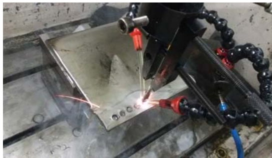
Figure 2 Experimental setup for machining of haste alloy C-276 (see online version for colours)
