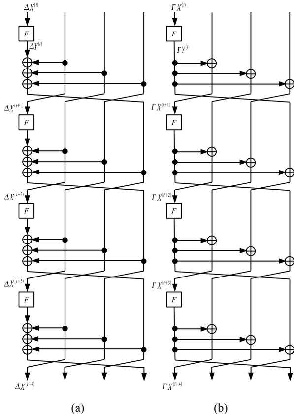
**Figure 6** p-Camellia block cipher structure
