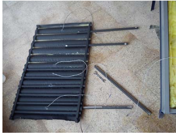
Figure 5 K-type thermocouple wires and tubes for PCM under the corrugated absorber sheet (see online version for colours)
