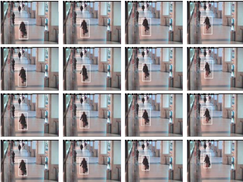
Figure 7 Results of edge feature fuzzy judgment and tracking of pedestrian with pedestrian tracking sequence woman (see online version for colours)
