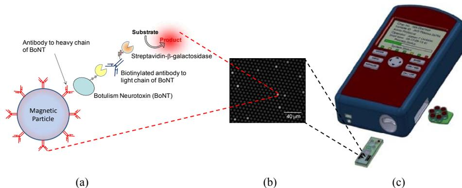
Notes: The bright wells correspond to a single enzyme label associated with a bead. All bead incubations, washing, array loading, and imaging occurs on a microfluidic chip. A handheld reader images the arrays, and a reagent cartridge houses beads and labelling reagents.
