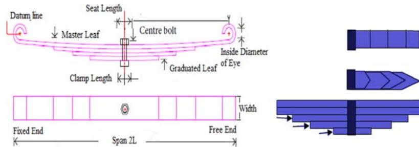
The specification of the vehicle model TATA LPT 1613TCIC truck is given in Table 3. The thickness and number of graduated leaves are modified in the proposed design and also the master leaf and the full length of first leaf thickness are changed but width dimension is maintained while designing. In this research, the Solidworks software package was used for CAD modelling of the leaf spring. The model was prepared as per the specification given in Table 3.
