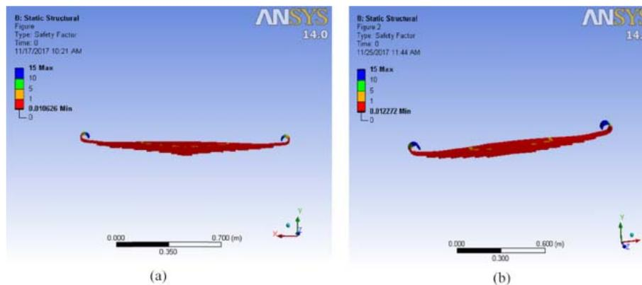
Table 6 shows the deflection and bending stress of the existing and the proposed model. The allowable safe stress determined between the corresponding loads is 2500 to 10,500 N; hence the near corresponding safe load is given in Table 6. From the table it was found that the maximum value of deflection and bending stress of the existing and modified models were compared with the results of the leaf spring. At the end of the
