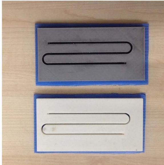
Notes: Channel-1 (above, grey) has a hydraulic diameter of 2.86 nm while channel-2 (below, white) has a hydraulic diameter of 1.67 nm.
