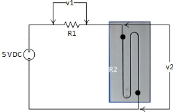
Notes: A low voltage supply would induce stress to the flooded channel ( $R_1$ ) so that how the fluid would respond to the electrical potential across it may be observed. There is a standard resistor ( $R_2$ ) connected in series with the channel. It works as a transducer that would confirm the existence of current flow in the circuit by measuring the voltage across it.
