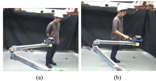
In these two experiments, the robot operates when the worker needs parts and/or a tool to complete the current task. After delivering the parts and the tool to the worker, the robot goes back to its home configuration and continues to wait there until the worker moves close to the next working position. In this experiment, we compare the results of the case without HRI constraints and the proposed scheme in two scenarios.
