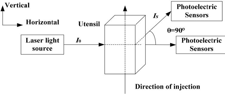
Using the theoretical basis of the scattered through ratio method, the measured liquid can be seen as separate pure fat thin solution and the same concentration of pure protein solution to study. So it can be seen as the laser was injected into the same concentration of pure fat dilute solution and the same concentration of pure protein solution (Zhou et al., 2006). According to Lambert's Law:
