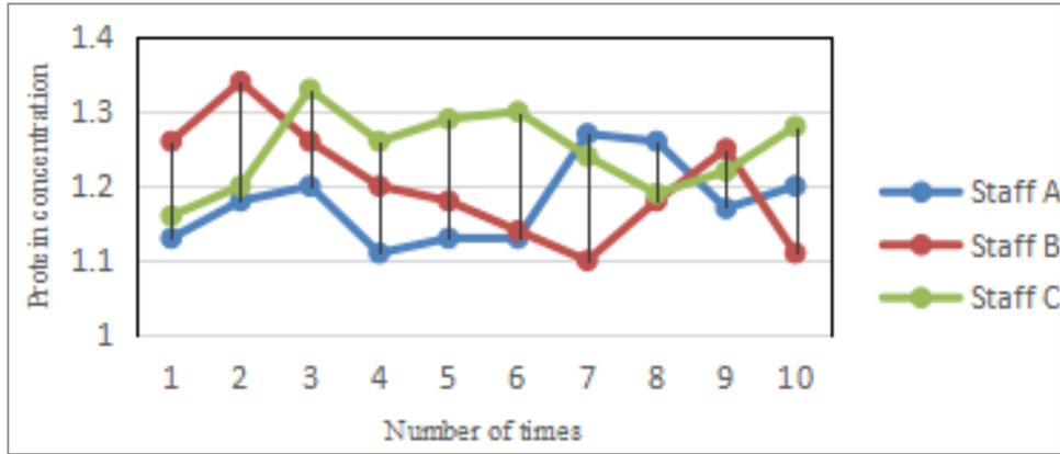
An analysis of multiple measured data yielded a measured concentrations average of A is 1.178, B is 1.212 and C is 1.247. After getting the average, we conduct uncertainty analysis of the results from multiple perspectives.
