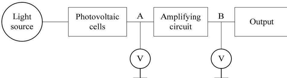
In the design of this module, the amplification part of the photoelectric detection circuit was tested and two photoelectric detection circuit boards were required due to receiving two signals of scattered light and transmitted light. So the two circuit boards were tested respectively. The test circuit is shown in Figure 7.
