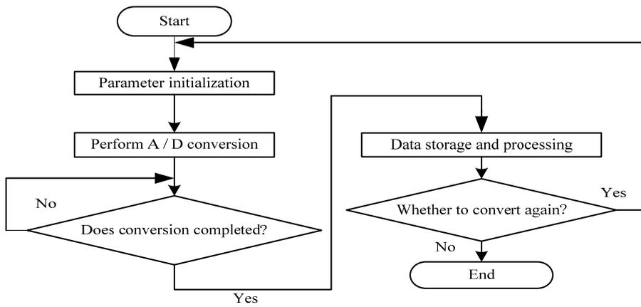
**Figure A4** The conversion diagram of ICL7135
