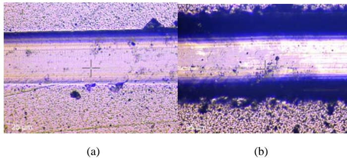
**Figure 7** Photographs of the scratch track in points corresponding to  $L_{c1}$  and  $L_{c2}$  for C type of coating (see online version for colours)
