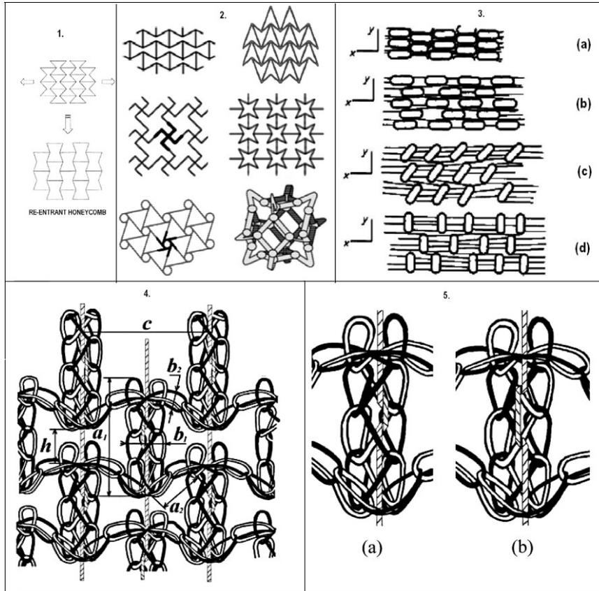
Notes: 1: Re-entrant honeycombs; 2: different forms of auxetic structures; 3: auxetic behaviour of laterally attached rods to polymers; 4 and 5: structure for auxetic textiles.
