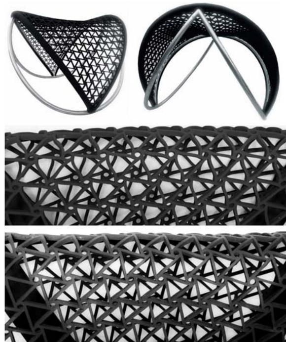
Note: Two views and a detail of the auxetic structure contracted and extended.
