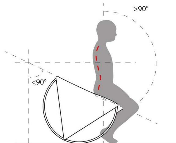
The material selected to realise the Chiral chair is water-jet cut neoprene to form the seat with auxetic texture and steel tube frames to realise the load-bearing structure. The main
