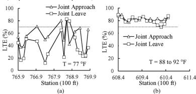
Figure 10 (a) Distressed section (EB) LTE and (b) control section (WB) LTE (100 ft = 30.5 m) (T = pavement surface temperature)
