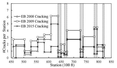
**Figure 5** Westbound cracking plot (100 ft = 30.5 m)
