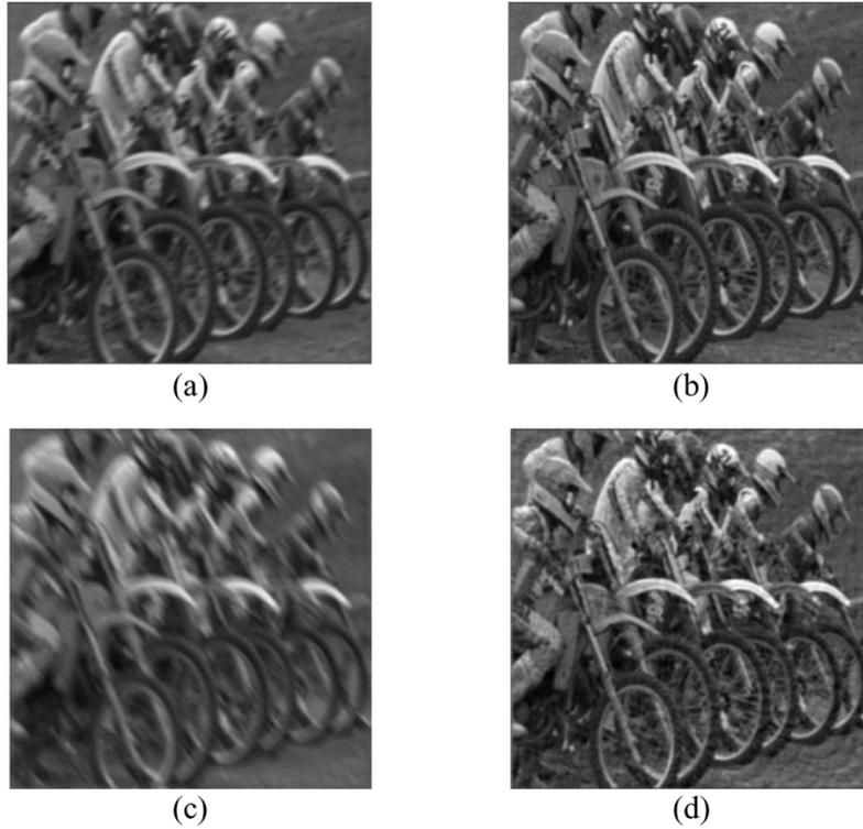
**Figure 4** Restoration outputs for colour image by motion blur parameters estimated from the proposed technique: (a) original image; (b) image blurred with motion blur of length 40 and angle 20 and (c) image (b) restored with estimated length 40.93 and angle 20.55 (PSNR = 26.2134 dB) (see online version for colours)
