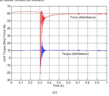
Figure 8 Performance of the RP robot with admittance and hybrid controllers, (a) end-effector force with admittance and hybrid controllers (b) end-effector position with admittance and hybrid controllers (c) joint torque and force with admittance controller (continued) (see online version for colours)
