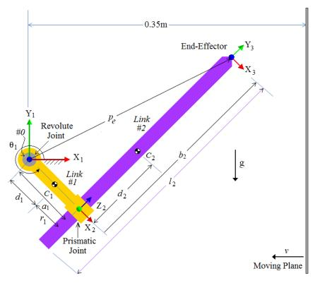
Figure 6 RP robot model (see online version for colours)
