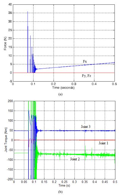
Figure 10 Performance of KUKA KR5 Arc robot with stiffness controller, (a) end-effector force (b) joint torques (see online version for colours)
