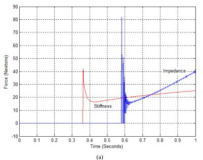
Figure 7 Performance of the RP robot with stiffness and impedance controllers, (a) end-effector force with stiffness and impedance controllers (b) end-effector position with stiffness and impedance controllers (c) joint torque and force with stiffness and impedance controller (continued) (see online version for colours)
