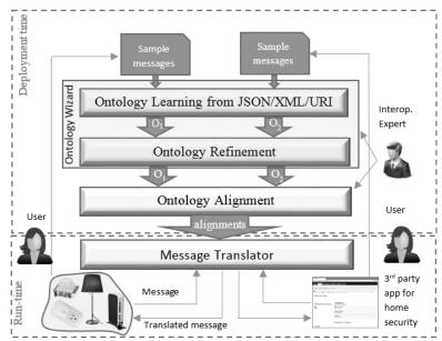
Figure 2 The smart proxy architecture instantiation for 'smart room' scenario
