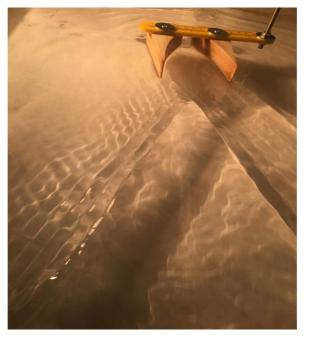
Figure 11 Flow pattern at the exit of the nozzle (see online version for colours)
