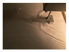
Figure 7 A bow shock is formed in front of a moving cylinder (see online version for colours)
