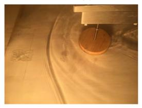
Figure 8 Flow over a cylinder with a sharp spike (see online version for colours)
