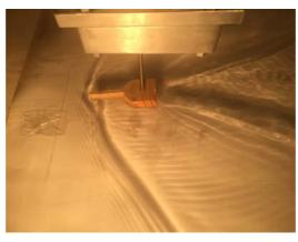
Figure 10 Shock formations inside the convergent/divergent nozzle (see online version for colours)
