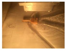
Figure 9 Shock pattern for flow around a cylinder with a spike (not so sharp) (see online version for colours)
