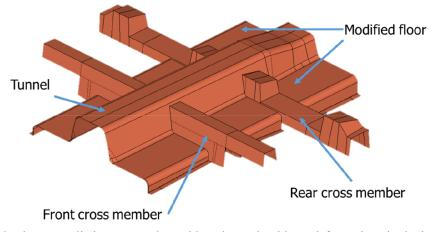
The load case applied corresponds to side pole crash with no deformations in the battery area allowed, i.e., the tunnel and modified floor area (Figure 5). The philosophy is that the steel structure for the normal car should not be changed in order to affect the overall assembly as little as possible. Energy absorption is assumed as taken up in the remaining steel floor structure.
