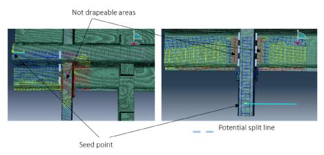
The draping analysis, in addition to split lines, also defines whether the part can be produced in one single preform, or if patching alternatively multiple preforms are required to realise the part.
