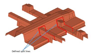
Figure 6 Proposed split lines due to the specific requirement for tunnel (see online version for colours)
