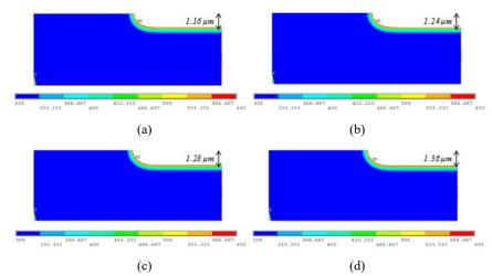
Simulated target profiles for laser fluence of, (a) 1 J/cm<sup>2</sup> (b) 1.5 J/cm<sup>2</sup> (c) 2 J/cm<sup>2</sup> Figure 8 (d) 2.5 J/cm<sup>2</sup> (see online version for colours)
