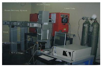
Figure 7 Photographic view of the experimental set-up (see online version for colours)
