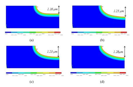
Figure 11 Simulated target profiles for curved surface ablation with various profiles, (a) uniform (b) Gaussian (c) parabolic (d) exponential (see online version for colours)
