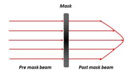
Figure 2 Modification of beam intensity profile using a mask (see online version for colours)
