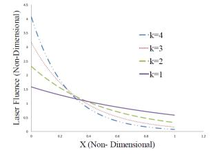
Figure 12 Exponential beam profiles considered for varying k (see online version for colours)
