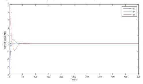
Based on Figure 4 to Figure 6, it can be found that the error angular velocity and error quaternion converges to zero. Except the initial 20 control cycles, the norm of control torque is constrained in an acceptable range.
