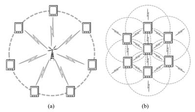
Figure 20 Wireless network configuration, (a) cellular model (b) mesh model
