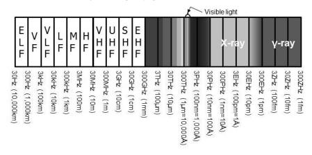
Figure 18 Radio (electromagnetic) frequency spectrum
