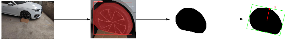
Figure 12 Failure to square the wheel (see online version for colours)
