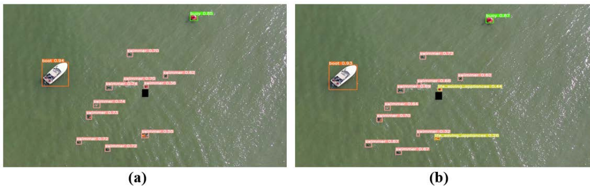
Figure 11 The fifth comparison of the model effects on maritime target detection before and after improvement, (a) YOLOv5s (b) YOLOv5s-NextSF (see online version for colours)
