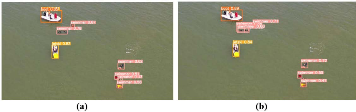
Figure 10 The fourth comparison of the model effects on maritime target detection before and after improvement, (a) YOLOv5s (b) YOLOv5s-NextSF (see online version for colours)
