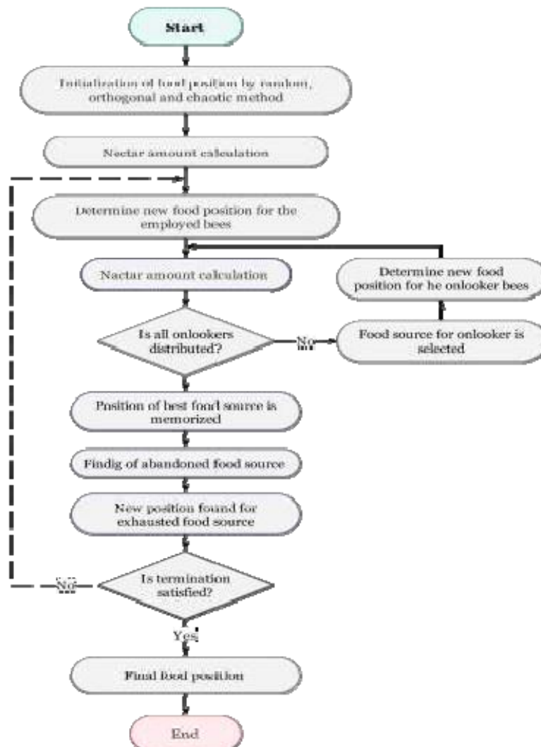
Figure 4 A flowchart illustrating the functionality of the ABC optimiser (see online version for colours)
