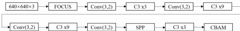
Figure 5 Structure of the backbone network after the addition of CBAM to YOLOv5
