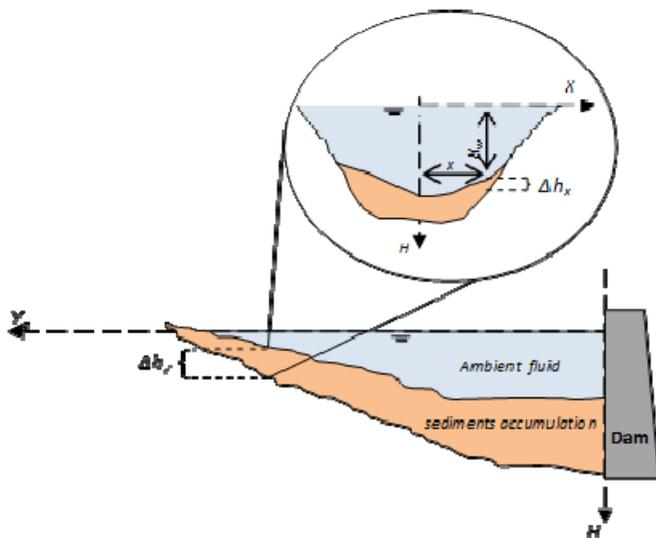
The concentration ( $C_s$ ) makes the difference between the density current, and the clear water density. This difference is a driving element of reservoir underflow (Cheng, 1997). The concentration was reduced along the reservoir until the dam, so according to the reservoir axis ( $Y_d$ ). However, the inertia of density current decreases from the reservoir entrance at the dam wall owing to the canal convergence. The current velocity reduces, which affects sedimentation intensity.
