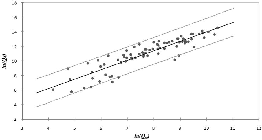
$$\ln(Q_{ms}) = 0.990 + 1.298 \ln(Q_{mw}) \text{ as } Q_{ms} = 2.691 Q_{ml}^{1.298}$$
