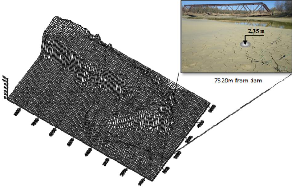
**Figure 4** Descriptive scheme of the sediment's accumulation variation along reservoir and in the cross sections (see online version for colours)
