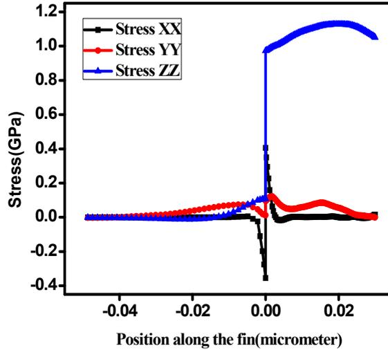
**Figure 6** Vertical stress profile in the device centre for a PFET device with  $\text{Si}_{0.8}\text{Ge}_{0.2}$  channel grown on  $\text{Si}_{0.9}\text{Ge}_{0.1}$  SRB (see online version for colours)
