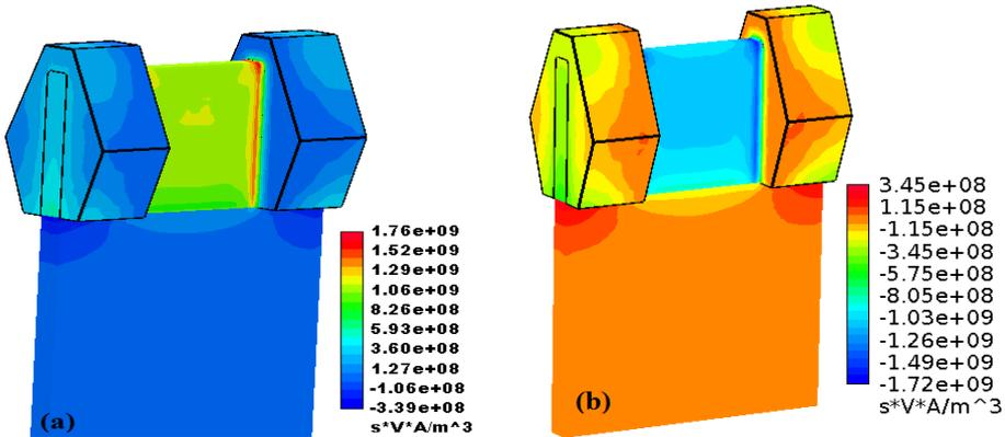
Note: The stress is generated due to lattice mismatch between the fin and S/D stressor.
