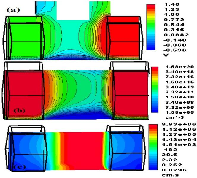
**Figure 8** Cut plane through the PFET device along the fin showing electrostatic potential, (a) hole concentration (b) average hole velocity (c) at  $V_{GS} = V_{DS} = -0.7V$  (see online version for colours)
