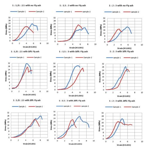
Figure 2 Stress-strain diagrams of the concrete cylinders (see online version for colours)
