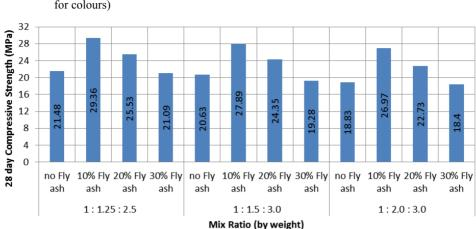
Figure 3 A comparative diagram for the compressive strength at 28 days (see online version for colours)
