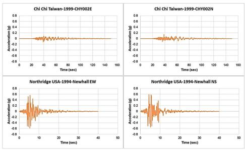
Figure 5 Horizontal acceleration records of the far-field (top) and near-field ground motions used in the study (see online version for colours)
