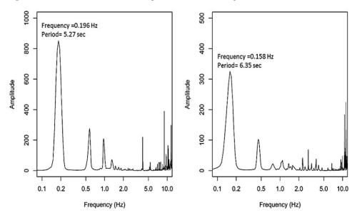
Figure 8 FFT of transfer function during the Loma Prieta earthquake
