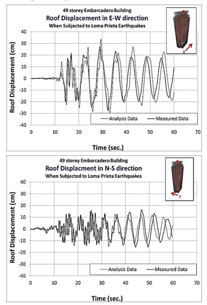
Figure 9 Roof displacement response of model and structures (see online version for colours)
