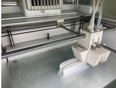
Figure 3 3D printing in Ultimaker S5 (colour) (see online version for colours)
