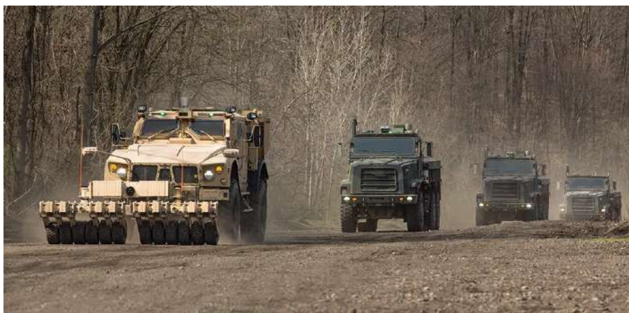
Figure 1 A typical vehicle equipped with a mine-rollers system (see online version for colours)
