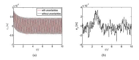
In Figure 9 we observe the robustness of the control where  $|e_a| = |\dot{x}_4 - \dot{x}_4|$  represents the acceleration deviation obtained by control without uncertainties  $(\dot{x}_4)$  and acceleration obtained by control with parametric uncertainties  $(\dot{x}_4)$ , and  $|e_u| = |u - \hat{u}|$  represents the signal control obtained by control without uncertainties (u) and signal control with parametric uncertainties  $(\hat{u})$ .
