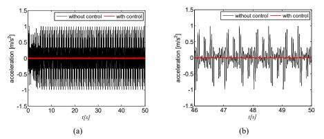
It is possible to observe that the proposed control reduces the system oscillation amplitude (Figure 5). The rms of the magnitude acceleration peak has been reduced in about 98.6367% (Figure 6), where the uncontrolled system acceleration ( $\ddot{x}_{3ms} = 0.2714$ )
