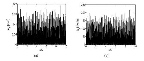
As can be seen in Figure 9, the proposed control is not sensitive to errors in the parameters of the matrix A, maintaining the level of acceleration and displacement below the uncontrolled system. As the acceleration in rms for the parametric error case is  $(\ddot{x}_{3ms} = 0.0449[m/s^2])$ , is possible to note that occurred a reduction of approximately (83.456%) relative to system without control, and the error was  $e_{3ms} = 1.0729 \times 10^{-7}[m]$  in rms.
